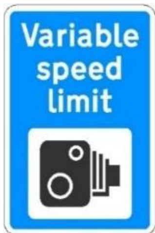
Variable speed limit with camera enforcement sign
